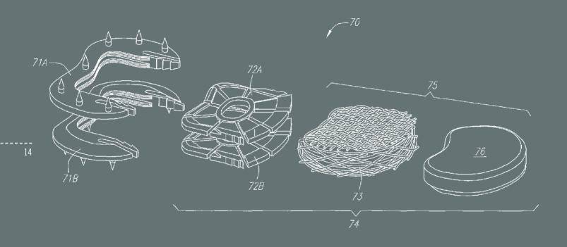
Curt Frank, the W. M. Keck, Sr., Professor of Chemical Engineering and director of the Center for Polymer Interfaces and Macromolecular Assemblies, helped develop a synthetic replacement for the intervertebral discs in the spinal column. The patented technology, illustrated above, has been licensed by Spinal Kenetics, founded in 2003.
