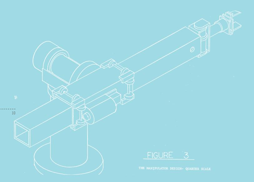
This illustration from the thesis of mechanical engineering graduate student Victor Scheinman, a pioneer in the field of robotics, shows the design of a computer controlled manipulator that became the model for later industrial robots.
